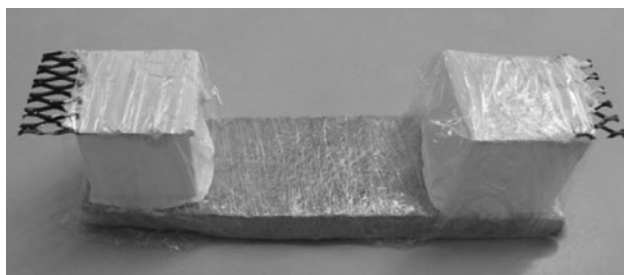
Fig. 3 Setup for electrokinetic desalination of tile segment. The electrode meshes were connected to the power supply
