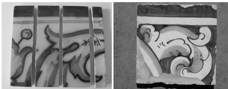
Fig. 2 a One of the XIX-century tiles used for the experiments (after segmentation). The thin slice at the right was a blind sample and the remaining slices were used for electrokinetic desalination experiments, b the salt damaged XVIII-a tile
